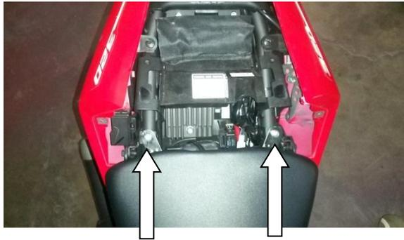
4) Remove the tool tray that is secured with two Philips pop rivets. Lift it out of the way
