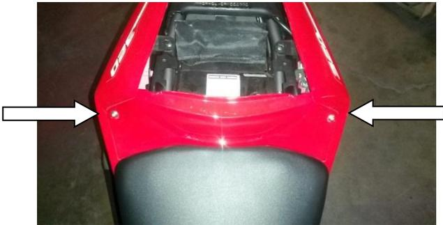
3) Remove the front seat by unscrewing the two 8mm bolts. Lift the seat out of place.
