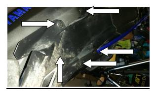
4)Pull the fairings out from around the OEM fender to expose the bolds securing it. A little steady pressure is required to do this as there are some clips holding it in place. Loosen the OEM fender(4) 8mm nuts from the bottom.
