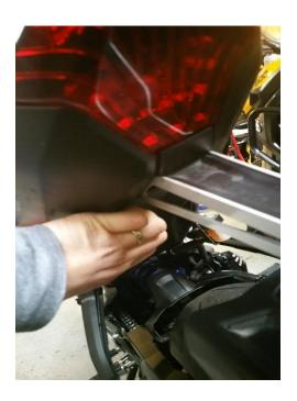
5) Trace back the OEM wires from the fender and disconnect them. There are two gray and one black connectors.
