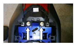
7) Swap out the (4) rubber garments and (2) screw clips from the OEM tail light to the new one. Install the new tail light and route the wires through the OEM route.
