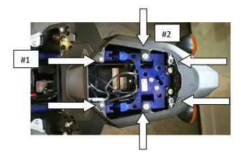
3) Remove the (5) pop rivets that are holding the plastic fairing around the OEM fender on the bottom.
