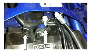
6) Remove the (2) 4mm Hex bolts holding the OEM tail light. Disconnect the triangular white tail light plug and remove the tail light.
