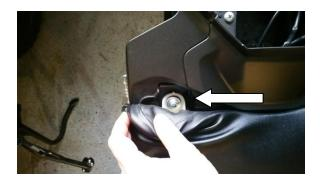
2) #1: Remove the front and rear covers around the back seat both held with (2) Philips screws. Pull the front cover up and the rear cover slides back and up. #2: remove the (2) 6mm Hex bolts securing the faring from the top(do not lose the spacers that are under these fairing bolts).
