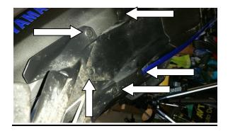
4)Pull the fairings out from around the OEM fender to expose the bolds securing it. A little steady pressure is required to do this as there are some clips holding it in place. Loosen the OEM fender(4) 8mmnuts from the bottom.
