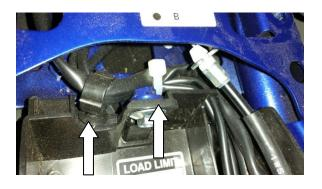
6) Feed the wires form your new fender eliminator through the wire opening from the bottom and attach the fender eliminator bracket with the (4) OEM 8mm bolts.
