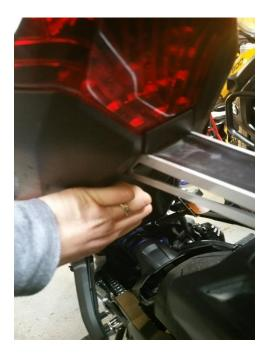
5) Trace back the OEM wires from the fender and disconnect them. There are two gray and one black connectors. Cut the zip tie securing the wires and undo the black clip next to it. Pull the wires out of the bike as you lower the OEM fender out of the way.
