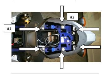
3) Remove the (5) pop rivets that are holding the plastic fairing around the OEM fender on the bottom.
