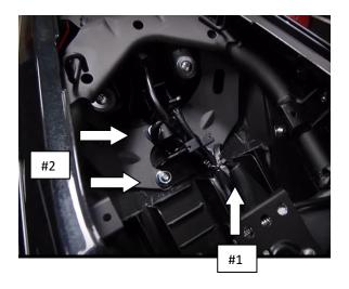
3) Install your new fender eliminator into the OEM location and secure it with the (4) OEM hex bolts and the nuts provided.
