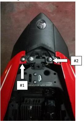
8) Remove the (6) Philips pop rivets on the bottom black fairing.
