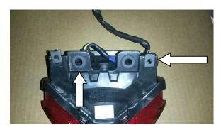
11) Install the new light into place by the same process the OEM light was removed. Reinstall the (2) 4mm Hex tail light bolts as well as the tail light cover and (2) screws that secure it.
