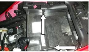
5) Unwrap the electric connectors that are protected by a clear insulator. Unplug the three electric connectors(round black and white, and rectangular white). Unplug the tail light wire.
