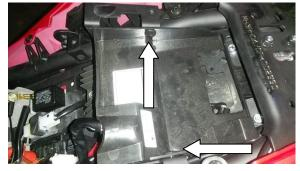
5) Unwrap the electric connectors that are protected by a clear insulator. Unplugthe three electric connectors(round black and white, and rectangular white ).
