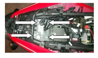
7) Install the new licenses plate bracket and feed the electrical cable through the opening and feed the cable into the original location. Use two OEM 10mm nuts and the two supplied bolts to secure the bracket(feed the bolts from the bottom).
