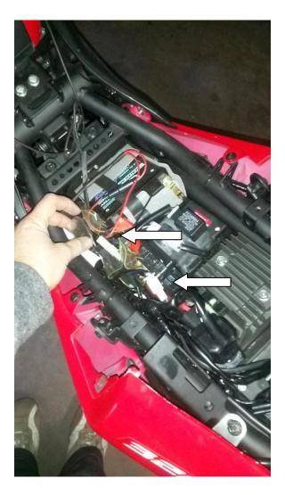
6) Remove the OEM fender: Unscrew the four 10mm nuts(you will reuse two of these to attach the new license plate bracket) and lower the fender out of the way as you pull out the 3 electrical cables. \*please note how they are routed in order to reinstall the new ones properly.
