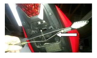
8) Route the wire bundle from the fender eliminator on the left side of the bike looking from behind and connect the electric connectors: 1)White connector 2) Gray plug to gray plug, black plug to black plug. 9)Reinstall the rest of the components in reverse order:
