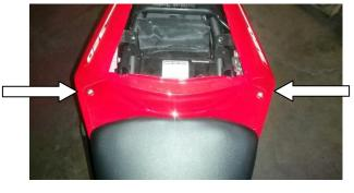
3)Remove the front seat by unscrewing the two 8mm bolts. Lift the seat out of place.
