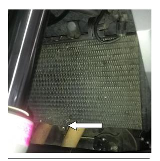
3) Position the radiator guard into place and adjust the nuts that are sitting against the radiator until the guard is flush with the radiator. Install nuts on the reverse side of the bolts and tighten all of them(using LocTite is recommended).
