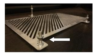
2) Remove the bottom T25 bolt on the radiator. There is an 8mm nut securing it on the reverse side.
