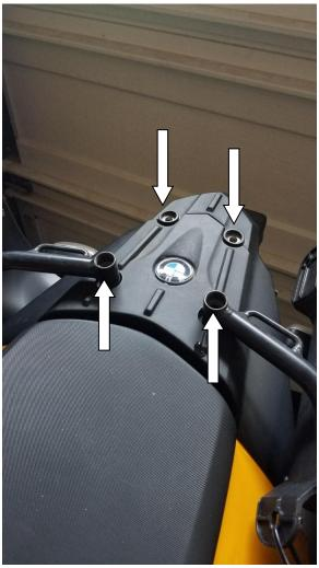
2) Position the (2) spacers provided over the rear holes and position the rack into place and
