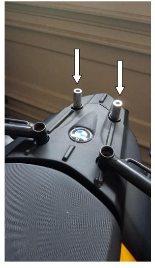
3) Bolt down the rack with the (4) T5 bolts provided.
