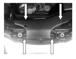
2) Feed the scoop through the left grill. Position the scoop in place, using a pencil mark where the holes for the screws must be drilled.
