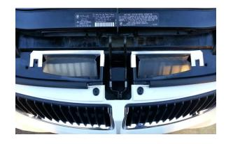
4) Place the intake elbow back into position and install the two lower clips making sure that they go through the slots in the scoops. Reinstall the two upper screws.
