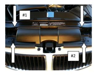
2) Insert the left hand side scoop diagonally into the left grill opening starting from the rear. You may need to apply slight pressure on the font corner of the scope in order to aid it into slipping into the opening. Repeat for the right hand side.
