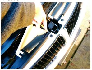
3)Position both the right and left scoops so that both the tab near the hood latch is in position as well as the outer scoop slot is aligned with the clip hole.
