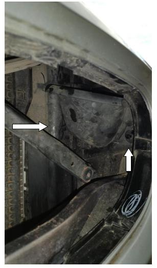
3) Feed the scoop through the opening into the right side grill and secure into place with the
