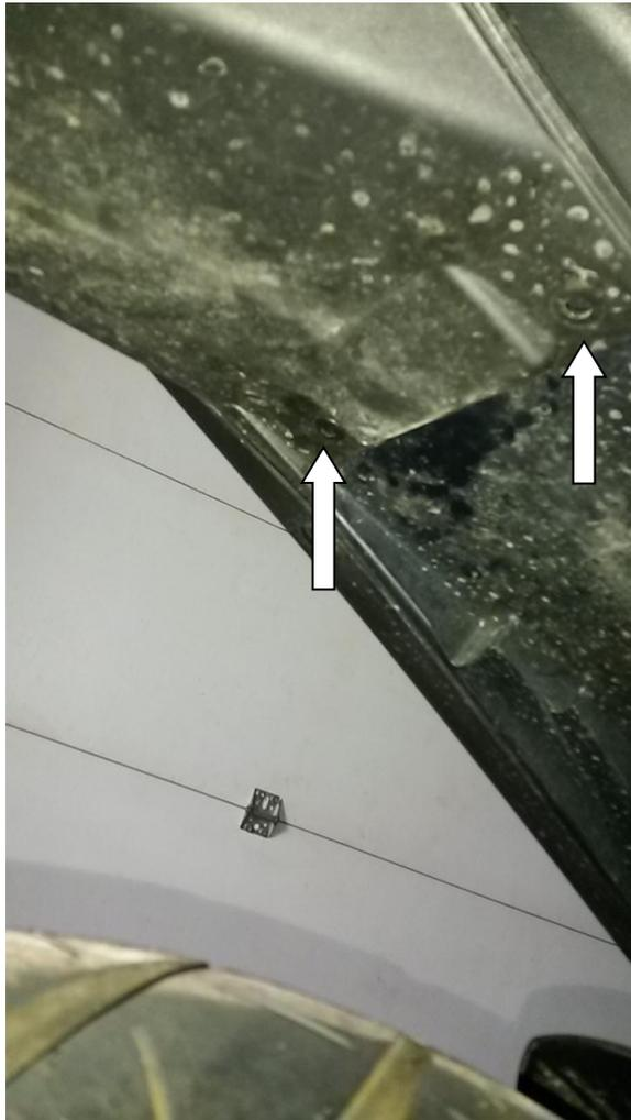
3) Remove the top tail light cover. It is secured with three screws. Slide it towards the back of the bike and remove.
