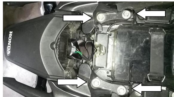
5) Remove the OEM fender. It is secured with:
