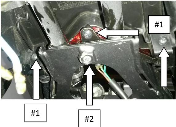
\*The bottom 12mm bolt is easiest removed by removing the bottom center tail light cover as shown:
