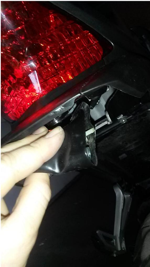
11) Remove the tape cover and position the AVT fender eliminator into place on top of the metal rear frame bracket and secure with one of the OEM 12mm bolts.
