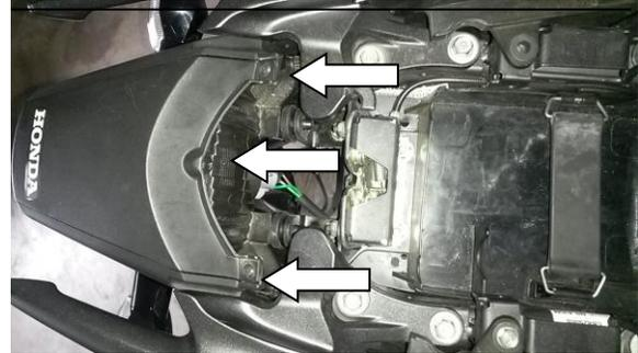
4) Remove the passenger handle bars by unbolting the (4) 12mm Bolts.
