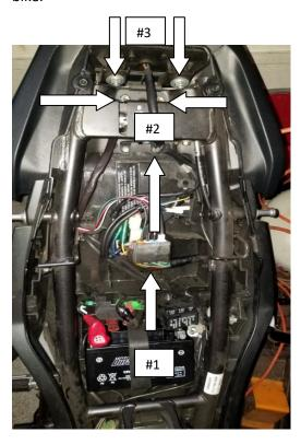
3) Route the fender eliminator wires into the bike from the bottom and secure the fender with (2) stock bolts and nuts provided. Reinstall the (2) tail light nuts.
