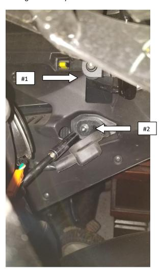
2) Remove the rubber garment that is in the fairings by pushing it out with a screw driver starting from the middle. You want it to come out towards the outside of the bike. Be careful not to damage anything as you do this.
