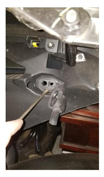
3) Slip on one of the provided spacers onto your new LED turn signal and feed the wiring through the fairing from the outside in. Slip another spacer onto the turn signal and secure with the nut.
