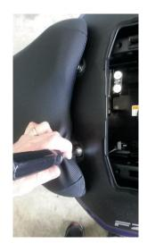
2) Loosen the OEM fender. You will need to remove: #1: (4) 13mm bolts from the top. #2 (2) push clips.
