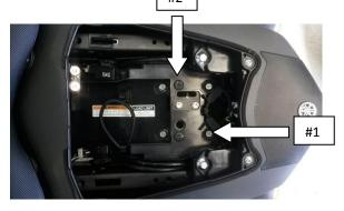
3) Trace back the wires from the fender and disconnect them.
