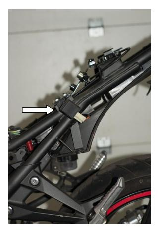
7) Remove the OEM Fender: 1) Unplug the four electric connectors. 2)Unscrew the four 5mm hex bolts.
