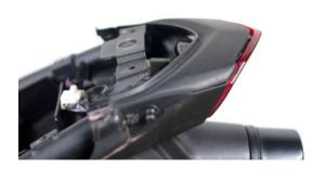
9) Remove the OEM tail light by unbolting the two 10mm bolts. You will reuse these bolts, the nut bracket that they screw into, as well as the rubber inserts from the OEM light to assemble your new LED tail light in the next step.
