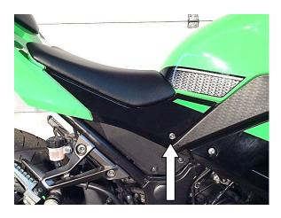
2)Remove the seat by unscrewing the two 5mm hex bolts(one on each side). Lift the seat out of place.
