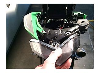
10)Install the upgraded LED tail light and feed the electrical wires through into the original location.
