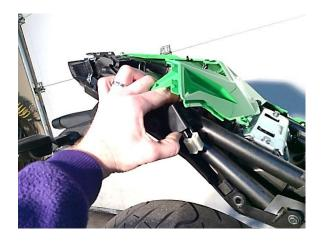
6) Remove the electric connectorsmetal protector plate by unscrewing the two 10mm bolts and lift it out of the way.
