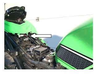
8) Remove the OEM fender: open up the storage tray that is under the rear seat and remove any items you may have in there.
