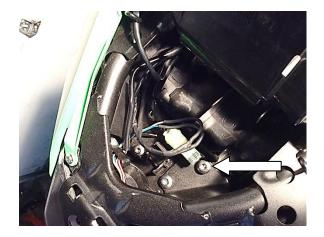
9) Remove the OEM tail light: on the rear of the light remove the three screws holding the tail light and pull it out from the rear with constant pressure. Pull out the electric wires along with
