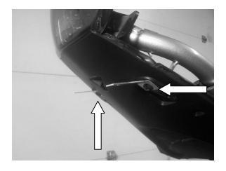
7) Attach the fender eliminator. First feed the wires through the opening, and route them back in the OEM location. Secure the fender eliminator with (2) of the supplied bolts and nuts. Once you have proper alignment of the fender eliminator and brackets tighten all of the bolts.
