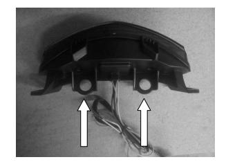
9) Connect the electric connectors: 1)white rectangular plug to black rectangular plug.2)orange plug to black plug 3) light blue plug to gray plug. Plug in the tail light connector.
