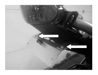
8) Take out the rubber inserts from the OEM tail light an install them in the same way into the LED tail light. Reinstall the new tail light.
