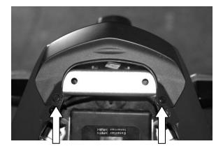
3) Remove the right and left rear fairings. They are secured with 2 pop rivets and one Philips screw. First pop out the front side of the fairing and then push it towards the rear of the bike to get it off.
