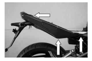
4) Unplug the four pictured electric harness under the rear right fairing(it may make it easier to figure out which ones to unplug by tracing back the wires from the OEM fender and tail light.
