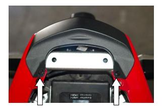
3) Remove the right rear fairing. It is secures with 2 pop rivets and one Philips screw. First pop out the front side of the fairing and then push it towards the rear of the bike to get it off.
