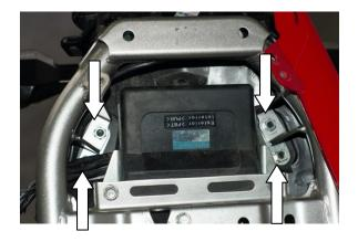
6) Attach the fender eliminator brackets with the (2)#25 torx bolts and nuts you just removed in the last step. Do not yet fully tighten the bolts.
