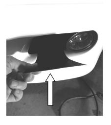
2) Once the scoop is past the bumper cover edge on the lower part of the opening, feed the scoop under the bumper cover as far as possible. 3) Reach in with your hands into the opening and position the snorkel side of the scoop into the air snorkel.
