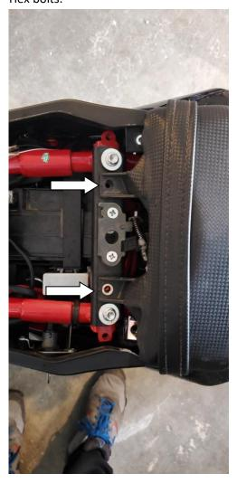
2)There is a wire that runs from the rear mud flap on the right side of the bike. Trace it from the back to where it plugs into the bike under the front seat on the right side by the frame. Unplug it and remove the wire until its fully free.
