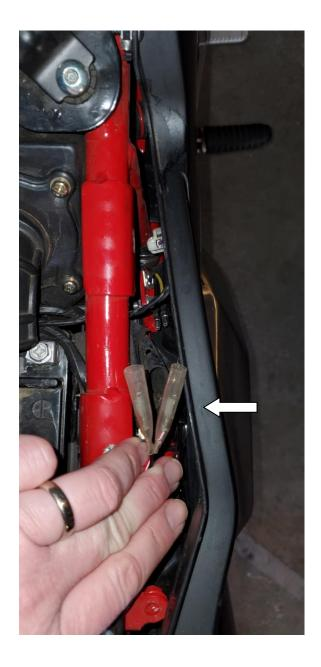
3) Remove the 4 bolts securing the mud flap((2) on each side) and lift it out of the way.
