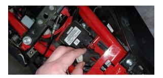
7) Secure the fender eliminator bracket with (2) OEM bolts and reinstall seats and the ECU plug if removed.
