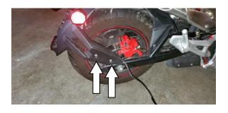
4)Remove the (3) OEM fender bolts.
