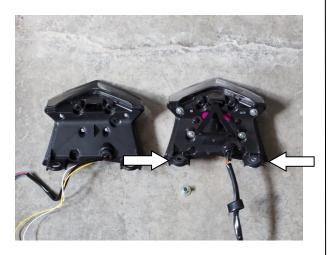
6) Install the integrated turn signal tail light into the OEM location and plug it in. Install your new fender eliminator bracket into the OEM location: Run the wires as they were with the OEM fender. Secure it with the (2) OEM hex bolts and the nuts provided.
