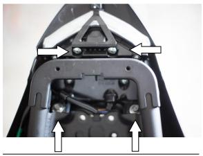
5) Unplug the tail light and remove it from the rear bottom fairing. Switch out the rubber gromets from the OEM light into your new integrated turn signal LED light.
