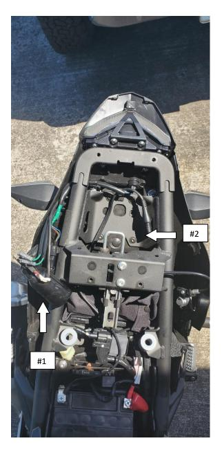
4) Remove the (2) Phillips screws that are on top securing the tail light followed by (2) 8mm
