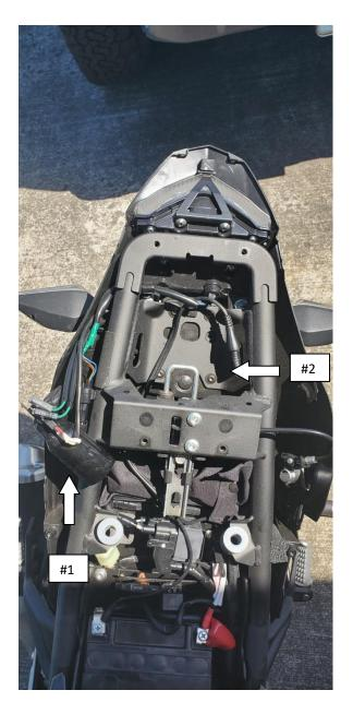
4) Install your new fender eliminator into the OEM location: Run the wires as they were with
