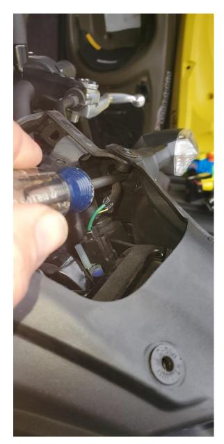
3) Once the Philips screw is removed the only thing that's holding the turn signal is two metal spacers. Pry these spacers out with a flat head screw driver and then twist the turn gingal out of the fairing.
