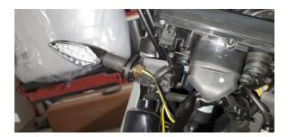
6) Plug in the turn signals pins into the supplied OEM connector as shown. Plug in the plugs and into the bike OEM orange and blue plugs.
