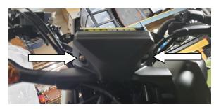
4) On the inside portion of the turn signal unscrew the nut. Remove the turn signal rubber garment that is in the fairings by prying out the metal insert with a screw driver starting from the middle. You will then want to grab the entire turn signal and twist it out of the fairing. A fair amount of pressure is needed.
