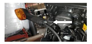
5) Install the new turn signal by placing one of the adapters onto the turn signal wiaring. Place the turn signal onto the fairing(where the oem turn signal was) and put an adapter on the other side and secure it with the nut.
