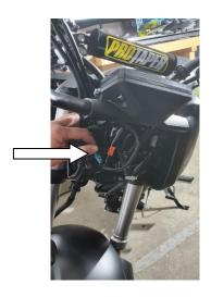
3) Remove the (2) hex bolts holding the turn signal fairing. Pull up on the fairing to remove it.
