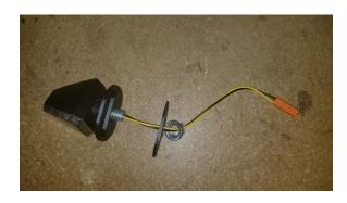
Plug in the turn signals and reinstall the two hex bolts holding the fairing. Ensure that the turn signals operate. If you also have rear LED turn signals you will need to add an LED rellay for the turn signals to work.
