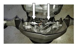
4) Install the new turn signal by placing one of the adapters with the protrusion onto the turn signal wiaring. Place the turn signal onto the fairing and put a flat adapter on the other side and secure it with the nut.
