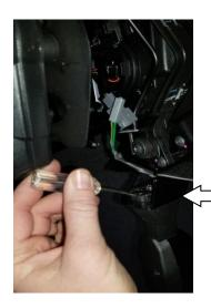
3) Unplug both turn signals and free the wiaring and remove the turn signals.
