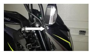
2) Remove the turn signal rubber garment that is in the fairings by prying out the metal insert with a screw driver starting from the middle. You will then want to grab the entire turn signal and twist it out of the fairing. A fair amount of pressure is needed but be careful not to crack the fairing.
