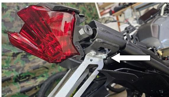
5) Remove the (4) 10mm bolts holding the top fairing bracket (by #2 in above diagram). Remove the (2) 4mm Hex bolts holding the tail light (by #5 in above diagram). Trace back the
