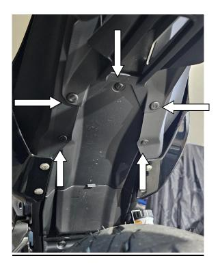
4)Pull the fairings out from around the OEM fender to expose the bolds securing it. A little steady pressure is required to do this as there are some pressure clips holding it in place. Pull out form the bike. Loosen the OEM fender (4) 8mm bolts from the bottom.
