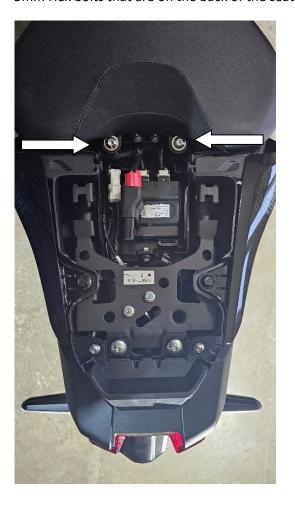
2) Remove fasteners holding the right and left rear fairings #1: (2) 4mm Hex bolts that are on the sides. #2: (2) 4mm Hex bolts. #3: (2) 12mm bolts under rubber grommets. #4: (2) 12mm bolts. #5: (2) 4mm Hex screws.
