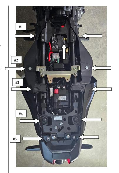
3) Remove the (5) pop rivets that are holding the plastic fairing around the OEM fender on the bottom. You press in the center to release them.
