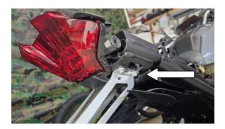
5) Remove the (4) 10mm bolts holding the top fairing bracket(by #2 in above diagram). Trace back the OEM wires from the fender and
