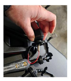
5) Feed the wires from the LED turn signal through the adapter and secure the turn signal as shown.
