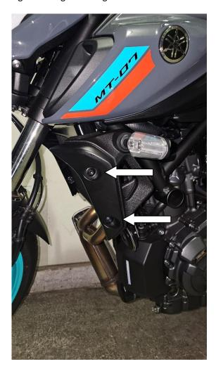
2) Follow the wires from the turn signals to find the connectors. Unplug both sides connectors. The left side is a little though to get to but can be unplugged with the aid of a small flathead screwdriver.
