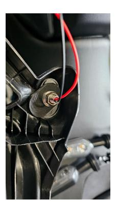
6) Plug the terminals of the turn signal wires into the plug adapter as shown. Red wire on the left. Black wire on the right.
