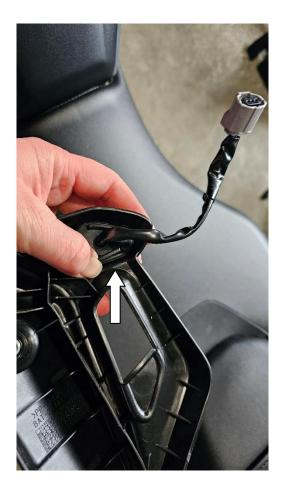
4) Position the provided adapter into the turn signal housing as shown.
