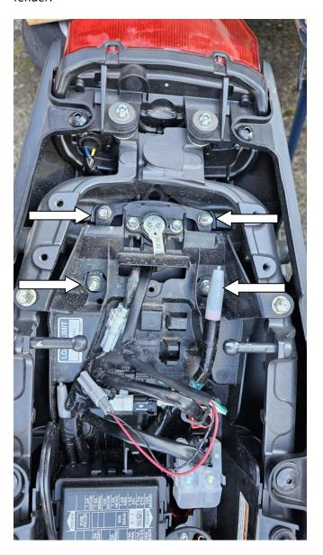
4) Trace the wires from the OEM fender to where they plug into the bike and disconnect the gray plug, black plug, and white plug.
