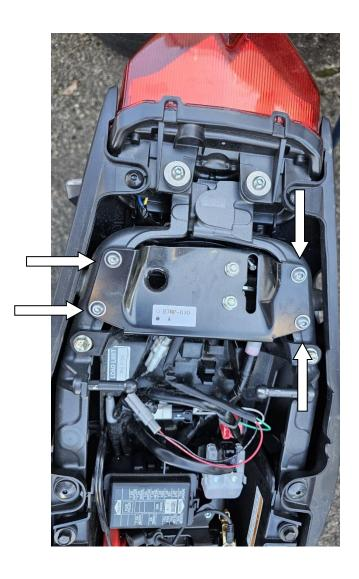
3) Remove the (4) 10mm nuts holding the OEM fender.
