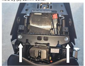
6) Remove the rear sear tray held by (2) pop rivets. Remove the electrical connector attached to the tray by pressing on the center. Remove the other electrical connector by pulling up and remove the tray.
