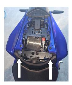
4) Remove the rear seat side fairings by removing (1) 10mm bolt (1) pop rivet on the side and (3) 10mm bolts on top. Slide the fairing out twards the back and out. Remove it on both sides of the bike.
