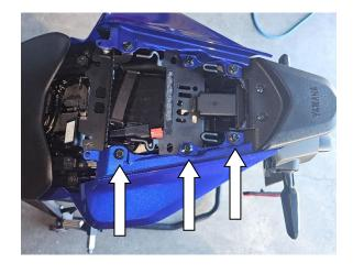
5) Remove the rear seat central metal bracket held by (2) 12mm bolts.
