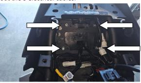
9) Install the new AVT licenses plate bracket and feed the electrical cable through the opening. Feed the cable into the original location. Use (4) OEM 10mm nuts and the (4) supplied bolts to secure the bracket(feed the bolts from the bottom).
