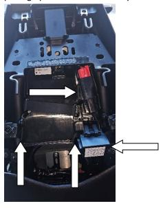
7) Pull up on the ECU and move it out of the way towards the front seat. There is no need to actual unplug it. Remove the rubber gromet around the fender wiring.
