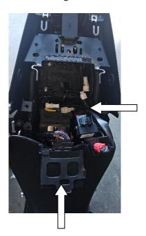
8) Unplug the 3 OEM fender plugs. (1) White, (1) Black, (1) Clear. Remove the OEM fender: Unscrew the (4) 10mm nuts(you will reuse these to attach the new license plate bracket) and lower the fender out of the way as you pull out the 3 electrical cables.
